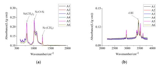
**Figure 4.** FTIR analysis results of samples under different years: (**a**) wave number between 500 and 2000 cm<sup>-1</sup>; (**b**) wave number between 2000 and 4000 cm<sup>-1</sup>.
