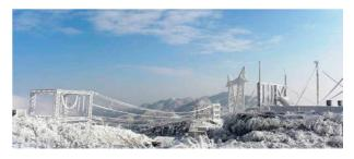
Figure 1. Aging environments of composite insulators in a high altitude area experimental station.
