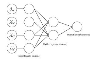
Figure 7. Structure of back propagation (BP) neural network.
