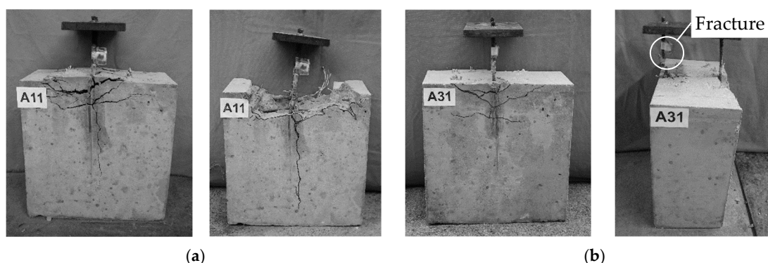
Figure 4. Cracks and failure patterns of specimens. (a) The crack and failure mode of A11; (b) The crack and failure mode of A31.
