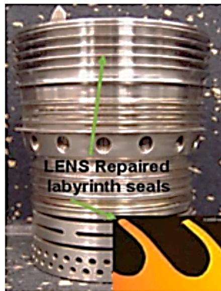
**Figure 13.** Gas turbine Inconel<sup>®</sup>718 compressor seal repaired by DED process [87].
