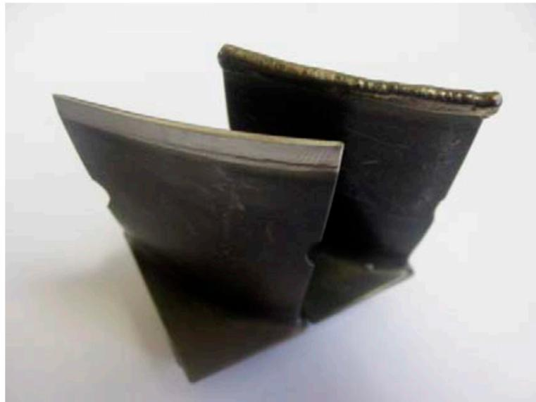
Figure 16. Thin-curved compressor blade before and after repairing [91].
