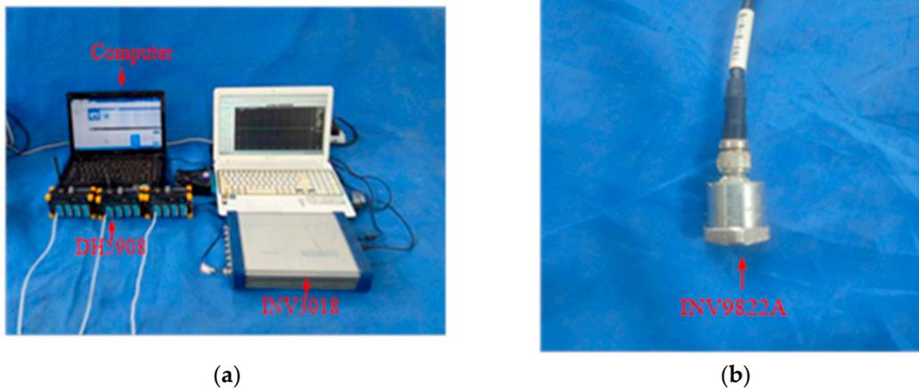
**Figure 8.** Test measurement equipment: (a) the Wireless Dynamic Strain Collector; (b) INV9822A accelerometer.
