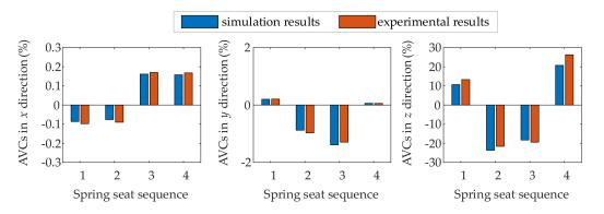
**Figure 14.** The amplitude variation coefficients (AVCs) of each spring seat in the *x*, *y*, and *z* directions under spring failure kind 5, including the simulation results and experimental results.
