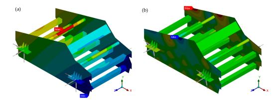
**Figure 4.** Vibration displacement contour map of the mining vibrating screen. (**a**) Overall vibration displacement contour map of the overall structure. (**b**) Lateral vibration displacement contour map.
