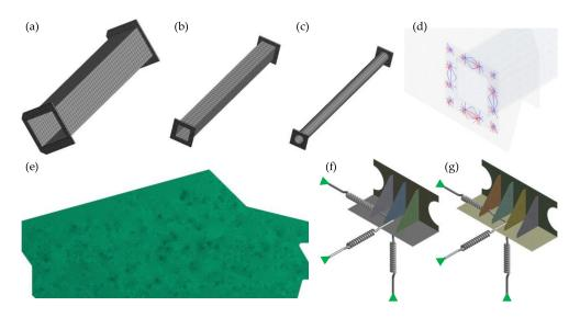
Figure 2. Meshed finite element model of the mining vibrating screen structures: (a) meshed exciting beam, (b) meshed bearing beam, (c) meshed reinforcing beam, (d) bolted connection, (e) meshed lateral plate, (f) loading side spring seat with simplified springs, and (g) unloading side spring seat with simplified springs.
