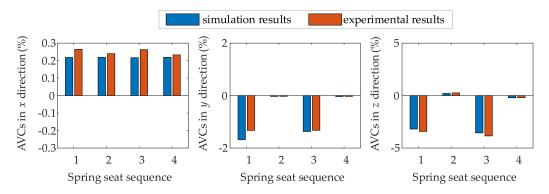
**Figure 13.** The amplitude variation coefficients (AVCs) of each spring seat in the *x*, *y*, and *z* directions under spring failure kind 4, including the simulation results and experimental results.
