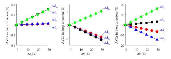
**Figure 6.** The amplitude variation coefficient (AVC) curves of each spring seat in the *x*, *y*, and *z* directions in the case of  $k_1$  failure.
