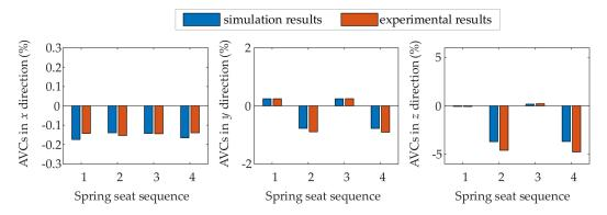
**Figure 15.** The amplitude variation coefficients (AVCs) of each spring seat in the *x*, *y*, and *z* directions under spring failure kind 6, including the simulation results and experimental results.
