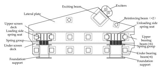
**Figure 1.** Structures of the SLK3661W mining vibrating screen (lateral view). The left side is the loading side and the right side is the unloading side.
