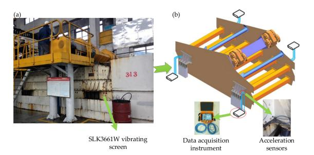
**Figure 8.** Experimental setup. (a) The SLK3661W vibrating screen applied in the coal washery. (b) Acceleration sensors and data acquisition instruments used in experiments.
