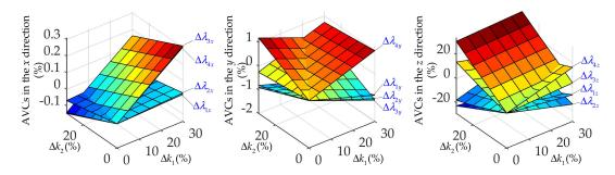
**Figure 7.** The amplitude variation coefficient (AVC) surfaces of four spring seats in the *x*, *y*, and *z* directions.
