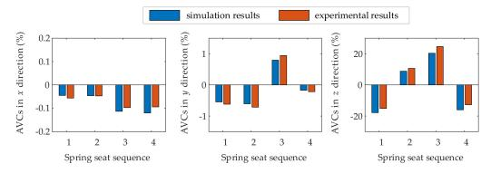
**Figure 11.** The amplitude variation coefficients (AVCs) of each spring seat in the *x*, *y*, and *z* directions under spring failure kind 2, including the simulation results and experimental results.
