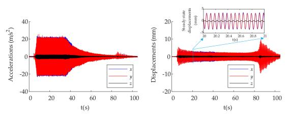
**Figure 9.** Acceleration and displacement curves in the x, y, and z directions of spring seat 2 under normal conditions, including the steady state displacement curves during 20–21 s.
