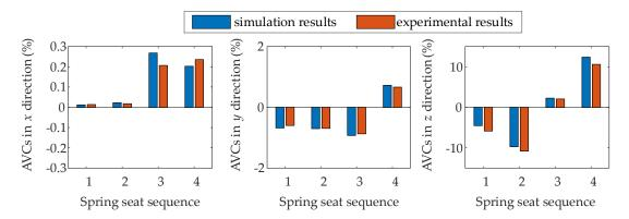
**Figure 10.** The amplitude variation coefficients (AVCs) of each spring seat in the *x*, *y*, and *z* directions under spring failure kind 1, including the simulation results and experimental results.
