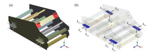
**Figure 3.** The overall finite element model of the mining vibrating screen. (**a**) POINT MASS units and alternating forces are applied on region A and region B. (**b**) Diagram of elastic supports.
