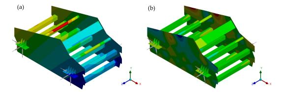
**Figure 5.** Vibration displacement contour map of the mining vibrating screen with spring failure. (a) Overall vibration displacement contour map of the overall structure. (b) Lateral vibration displacement contour map.
