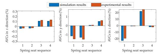
**Figure 12.** The amplitude variation coefficients (AVCs) of each spring seat in the *x*, *y*, and *z* directions under spring failure kind 3, including the simulation results and experimental results.
