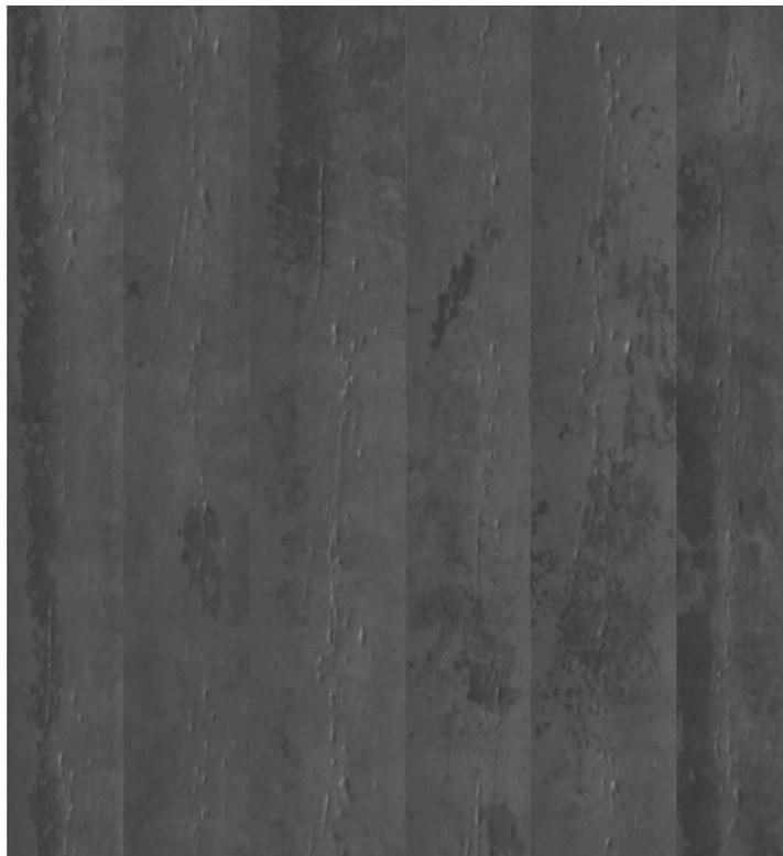
**Figure 3.** Roll marks on different batches.
