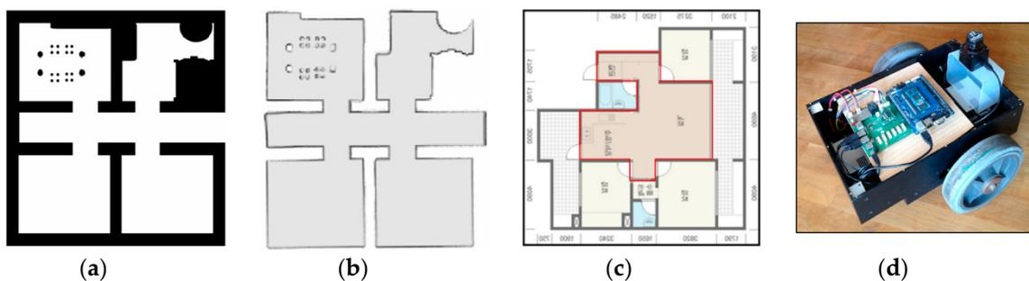
**Figure 8.** The experiment environments. (a) The simulated environment using player/stage; (b) The grid map produced by DP-SLAM for (a) environment; (c) The real environment; (d) The robot the authors built.
