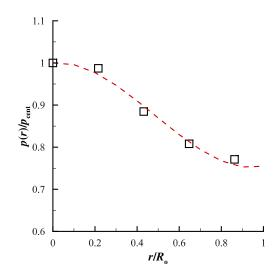
**Figure 6.** Distribution of the pressure for the E = 1.1 kPa silicone disk as a function of radial position with a 3<sup>rd</sup>-order polynomial fit overlaid. The polynomial fit is given by  $p(r)/p_{cent} = 0.6438(r/R_o)^3 - 0.9412(r/R_o)^2 + 0.04751(r/R_o) + 1.0$ .
