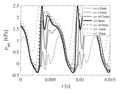
**Figure 15.** Intraglottal pressure waveforms as a function of pressure transducer position, acquired at  $p_{sub} = 2.15$ kPa. Superiorly increasing transducer locations are denoted by decreasing grayscale values for the solid lines, and a postive *x* position. Inferior positions are denoted by decreasing grayscale values for the dashed lines, and a negative *x* position.
