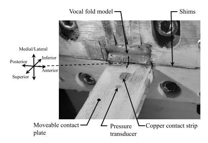
**Figure 10.** A close-up view of the hemi-vocal fold configuration, with the moveable contact plate. The location of the copper strip for measuring contact and the embedded pressure transducer are also noted.
