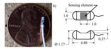
**Figure 2.** (a) Photograph of the Millar Mikro-Cath<sup>™</sup> pressure transducer from a top view. (b) Schematic of the top and side views of the pressure transducer geometry and dimensions. Dimensions are shown in mm.
