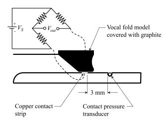
Figure 11. Schematic drawing of the hemi-vocal fold orientation and the Wheatstone Bridge circuit utilized for locating the point of contact.
