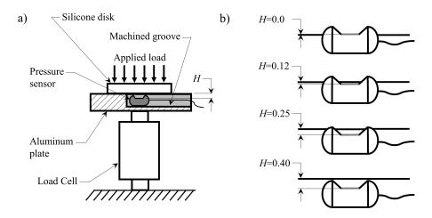
**Figure 3.** (a) Schematic of the custom facility for characterizing the pressure transducer performance in conditions representative of vocal fold contact. (b) Orientation of the pressure sensor relative to the surrounding contacting surface at the 4 sensor depths that were investigated. Dimensions are shown in mm.
