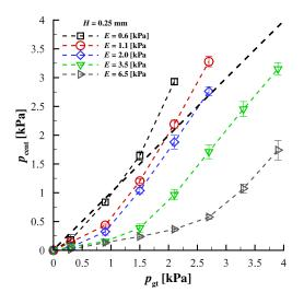
**Figure 5.** Variation of the pressure at the center of the contacting silicone disk as a function of the modulus of elasticity of the disk, for an offset distance of H = 0.25 mm (see Figure 2). The line of one-to-one correspondence between the measured and ground truth pressure is denoted by the heavy, dashed, straight line. The symbols denote the mean value and the bars indicate the maximum and minimum values for each trial.
