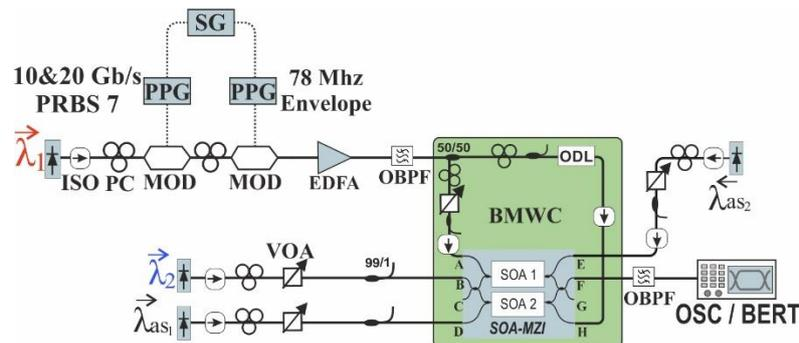
**Figure 1.** Experimental setup for testing the proof of concept of the Burst-Mode Wavelength Converter (BMWC). EDFA: Erbium Doped Fiber Amplifier; ISO: Isolators; MZI: Mach Zehnder Interferometer; OBPF: Optical Bandpass Filter; PC: Polarization Controllers; PPG: Programmable Pattern Generators; PRBS: Pseudo Random Bit Sequences; SOA: Semiconductor Optical Amplifier; VOA: Variable Optical Attenuators.
