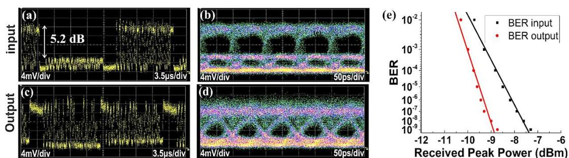
**Figure 5.** Experimental results for 10 Gb/s packets and 25 km fiber transmission (a) input trace (3.5  $\mu$ s/div), (b) input eye diagram (50 ps/div) (c) BMWC output trace, (d) BMWC output eye diagram and (e) BER measurements without the BMWC (input) and with the BMWC (output). All traces and eyes are in 4 mV/div.
