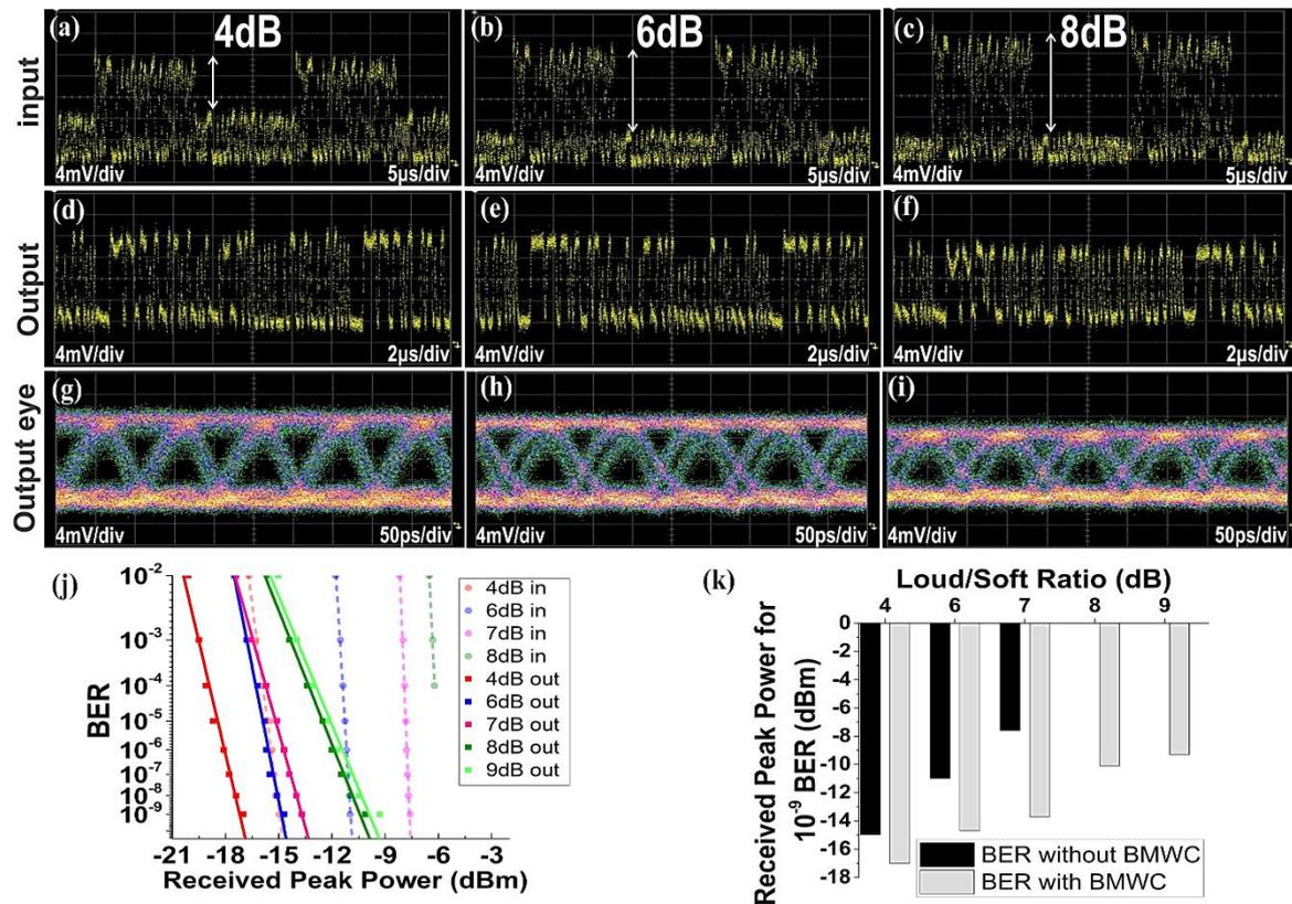
**Figure 2.** Experimental results for 10 Gb/s for 4 dB loud/soft ratio (a) input trace (5 μs/div), (d) output trace (2 μs/div), (g) output eye diagram (50 ps/div). For 6 dB (b) input trace, (e) output trace, (h) output eye diagram. For 8 dB (c) input trace, (f) output trace, (i) output eye diagram, (j) Bit Error Rate (BER) measurements for input and output signals and (k) BER improvement of input–output signals at different loud/soft ratios. All traces and eyes are in 4 mV/div.
