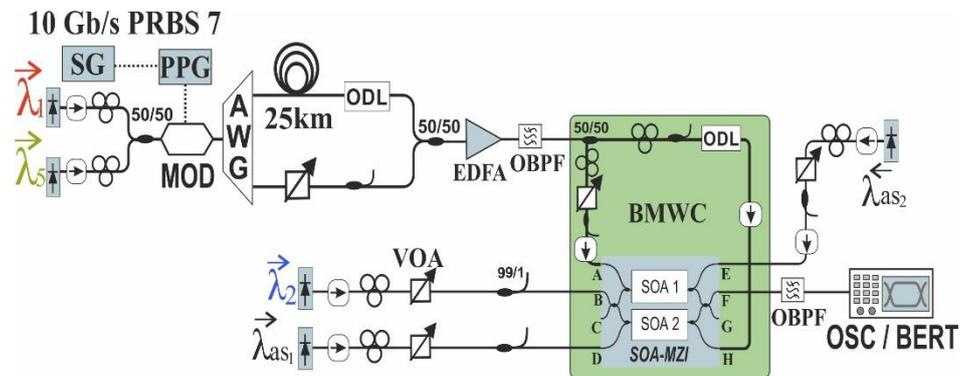
**Figure 4.** Experimental setup for testing the BMWC with 25 km fiber transmission. AWG: Arrayed Waveguide Grating.
