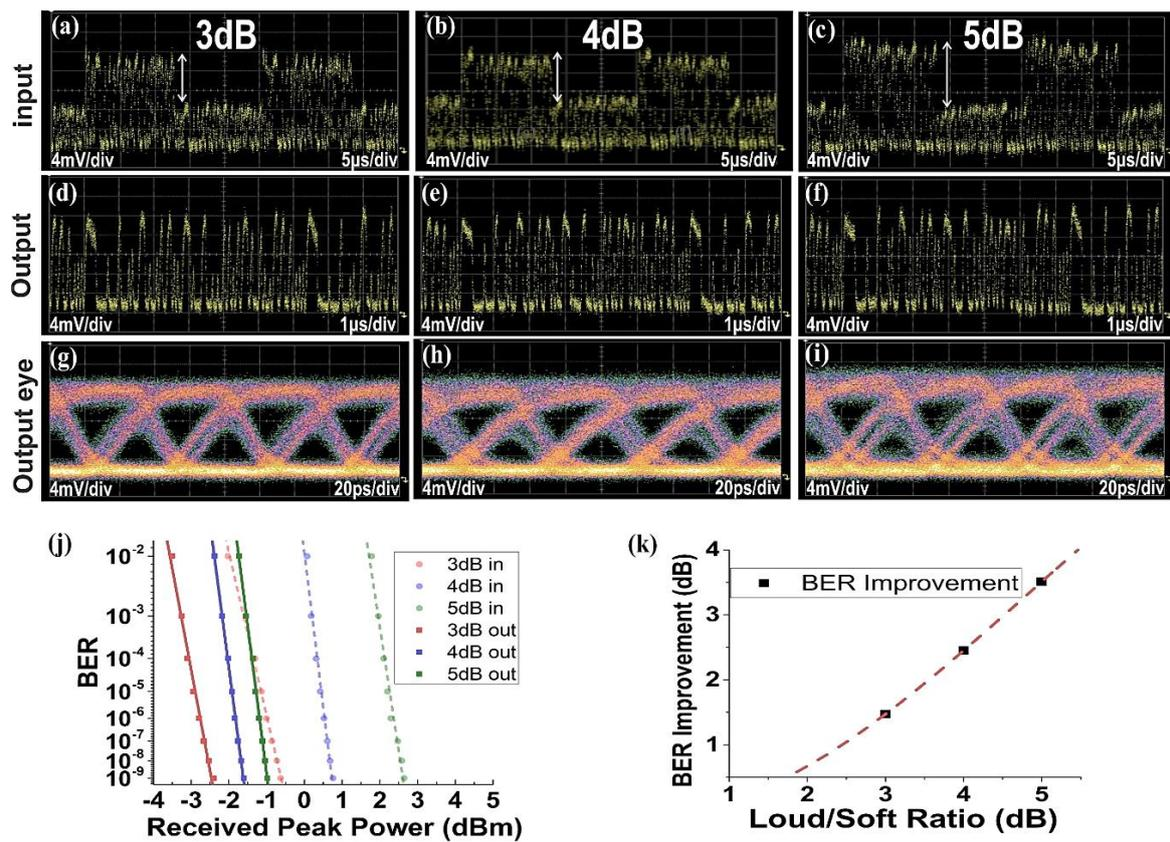
**Figure 3.** Experimental results for 20 Gb/s for 3 dB loud/soft ratio (a) input trace (2.5 μs/div), (d) output trace (1 μs/div), (g) output eye diagram (20 ps/div). For 4 dB (b) input trace, (e) output trace, (h) output eye diagram. For 5 dB (c) input trace, (f) output trace, (i) output eye diagram, (j) BER measurements for input and output signals and (k) BER improvement of input-output signals at different loud/soft ratios. All traces and eyes are in 4 mV/div.
