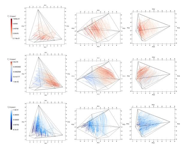
**Figure 6.** The trajectory patterns of the time-averaged principal strain-rates: averaged first principal strain-rate (**top**); averaged second principal strain-rate (**middle**); and averaged third principal strain-rate (**bottom**). In these graphs, the red color is used to represent extension, while the blue color depicts contraction.
