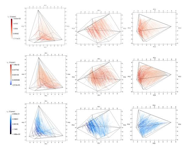
**Figure 5.** The trajectory patterns of the principal strain-rates at the year 2003: first principal strain-rate (**top**); second principal strain-rate (**middle**); and third principal strain-rate (**bottom**). The color scale in these graphs determines the strain type: the red color is used to represent extension, while the blue color depicts contraction.
