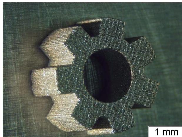
**Figure 9.** Final result of the 3D printed wick.
