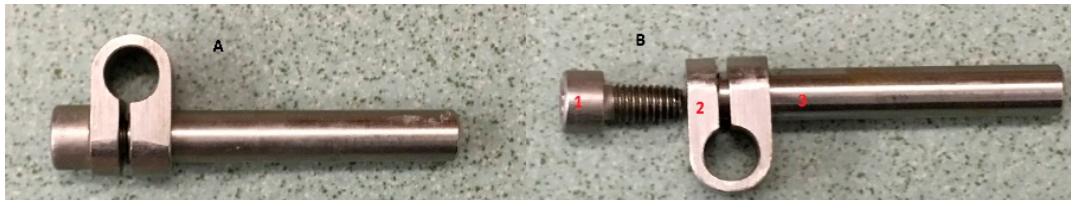
Figure 2. Arm and its elements: (A) Mounted arm; (B) parts of the arm; (1). M5 screw, (2) clamp, (3) rod.
