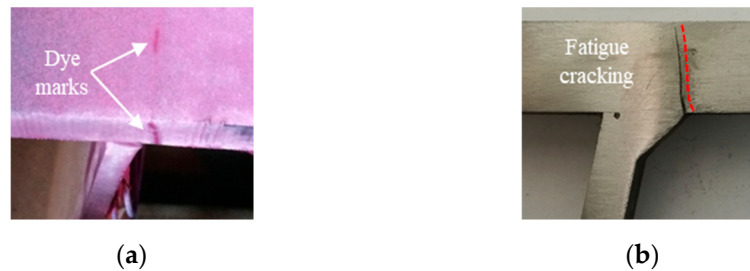
Figure 2. Typical cracking pattern: (a) Crack identified by DP checks; (b) Macro-section of the cracked joint.
