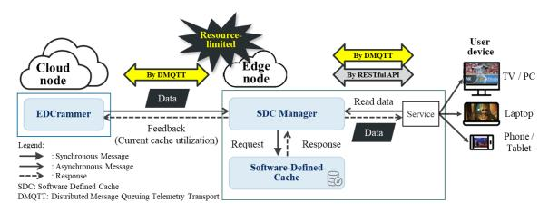
Figure 3. A communication diagram illustrating the interface between entities.
