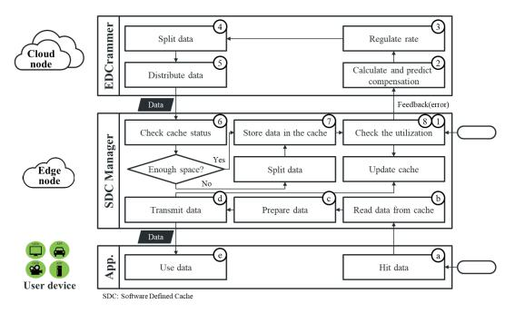
Figure 4. Overall flow for the data caching and hitting process.
