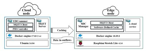
Figure 7. Performance evaluation environment for EDCrammer-based caching.
