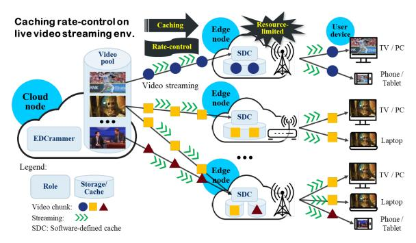
Figure 2. A concept of efficient edge caching between a cloud and edge nodes for live video streaming.
