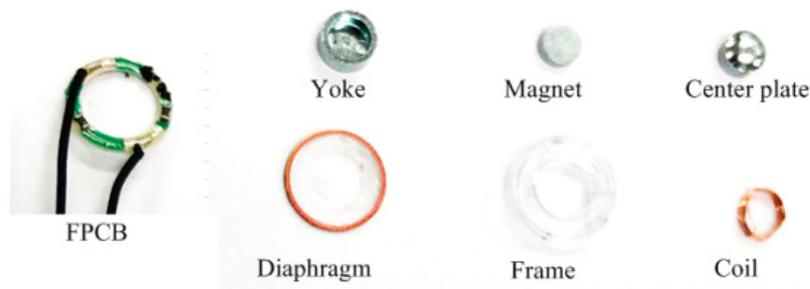
Figure 22. Components of dynamic earphone.
