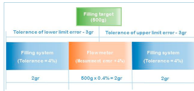
Figure 2. Filling error analysis for filling targets.
