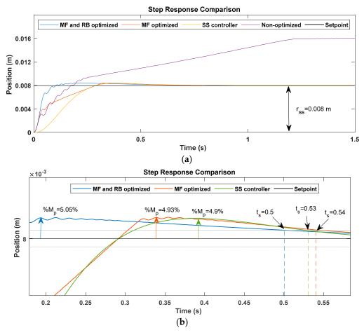
**Figure 7.** Fuzzy logic control of the MLS (MLS-FLC) with only MF's positions optimized, with membership function (MF) and rule base (RB) optimized, non-optimized and MLS with state-space (SS) controller step response: (**a**) Steady-state response, (**b**) dynamic response.
