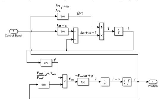
Figure 2. MLS model representation in Simulink.
