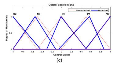
**Figure 6.** Optimized and non-optimized MF used for inputs and output data: (**a**) Position error (input), (**b**) derivative of error (input), (**c**) control signal (output).
