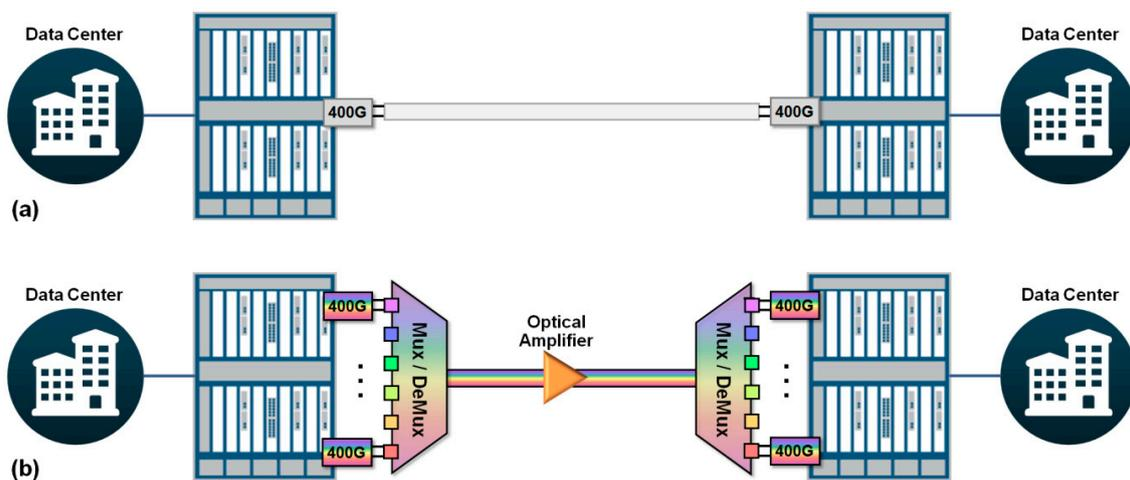
**Figure 1.** Typical application scenarios of 400 Gb/s pluggable optics for data center interconnect. (a) Unamplified point-to-point applications for 40 km reach; (b) amplified dense wavelength division multiplexing (DWDM) applications for 80–120 km reach.
