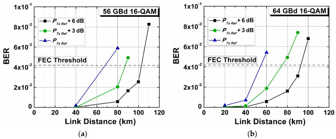
Figure 5. Bit error ratio (BER) as a function of transmission distance in unamplified point-to-point link for (a) 56 GBd 16-QAM signals; (b) 64 GBd 16-QAM signals.
