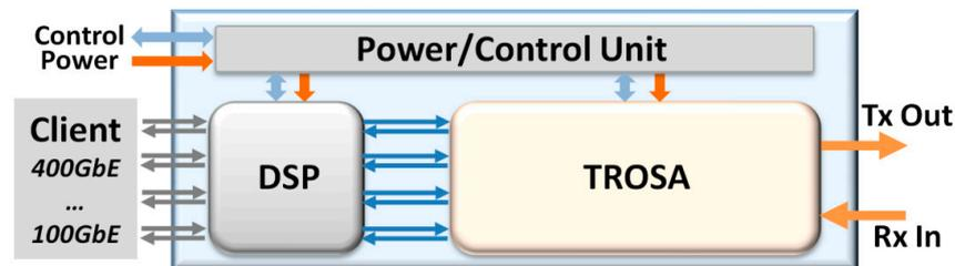
**Figure 3.** Typical architecture of 400G pluggable coherent transceiver. DSP: digital signal processing, TROSA: transmitter and receiver optical subassembly, Tx: transmitter, Rx: receiver.
