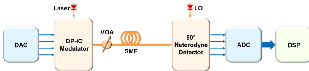
**Figure 4.** Experimental setup. DAC: digital-to-analog converter, IQ: in-phase (I) and quadrature (Q), VOA: variable optical attenuator, SMF: single-mode fiber, LO: local oscillator, ADC: analog-to-digital converter, DSP: digital signal processing.
