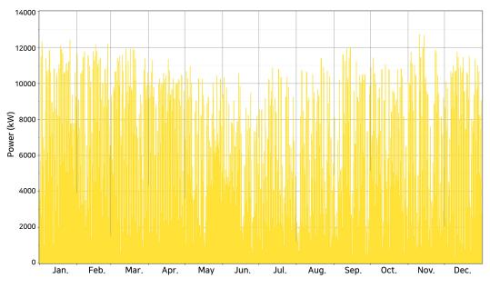
Figure 8. Monthly PV power production of the suggested configuration (created by the authors).
