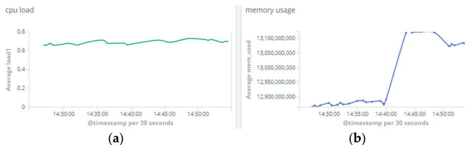
**Figure 11.** Visibility data collection overhead for packet-precise network flows. (a) CPU load and (b) memory utilization.
