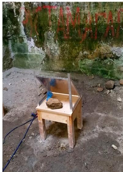
**Figure 3.** One of the nuclear emulsion detectors mounted inside the object at a depth of about 10 m at an angle of  $45^\circ$  in the direction of a wall.
