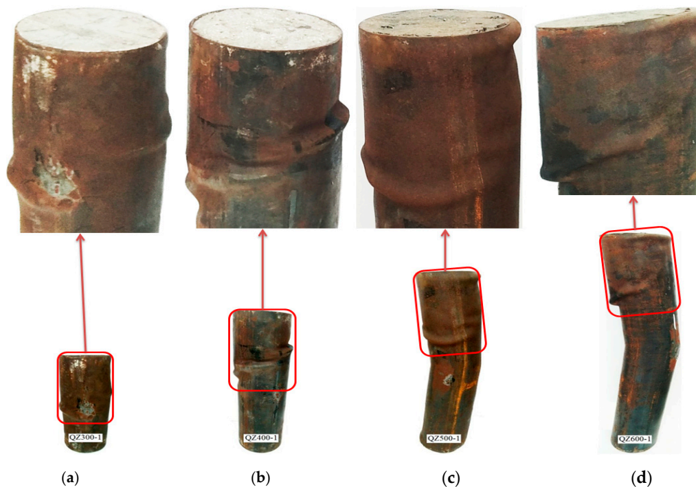
Figure 4. Failure mode: (a) \lambda = 2.6 ; (b) \lambda = 3.5 ; (c) \lambda = 4.4 ; (d) \lambda = 5.3 .
