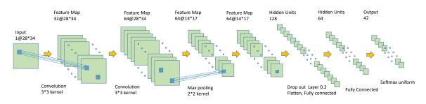
Figure 6. The architecture of a character recognition CNN.
