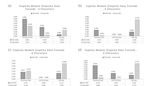
**Figure 10.** Test Results of Individually Trained Modules. (**a**,**b**) Only Claptcha data are trained to validate Claptcha and Captcha modules respectively. (**c**,**d**) Only Captcha data are trained to validate Claptcha and Captcha modules respectively.
