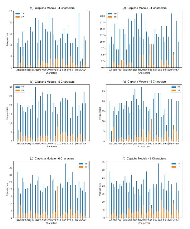
Figure 9. Statistics of True Positive and False Positive over Different Types of Testing CAPTCHAs.
