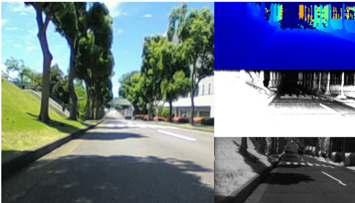
**Figure 4.** Example of outputs of the prototype LiDAR sensor with a reference image in an outdoor environment: **(top right)** range data; **(middle right)** peak intensity data; **(bottom right)** monocular data. Left figure shows reference image obtained by a camera.
