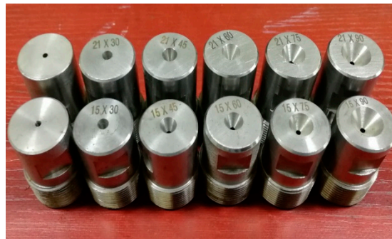
Figure 4. Picture of the tested organ-pipe nozzles.
