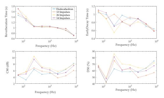
Figure 11. RT, EDT,  $C_{80}$  and  $D_{50}$  measured with different speaker placement methods.
