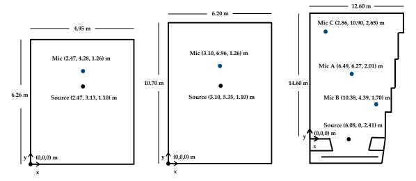
**Figure 1.** Source and microphone positions for the three spaces with volumes of 88 m<sup>3</sup>, 192.4 m<sup>3</sup> and 1088 m<sup>3</sup> (from **left** to **right**) where measurements were performed.
