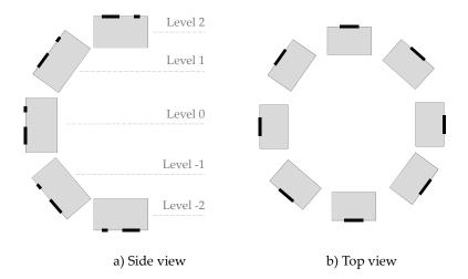
Figure 4. Side (a) and top (b) view for the measurements with a total sum of twenty six positions.
