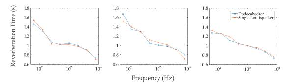
Figure 8. RT for points A, B and C in the amphitheater (from left to right respectively).
