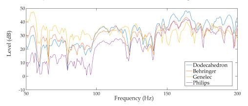
**Figure 13.** Frequency responses for measurements with the dodecahedron speaker and the proposed method with different speakers.
