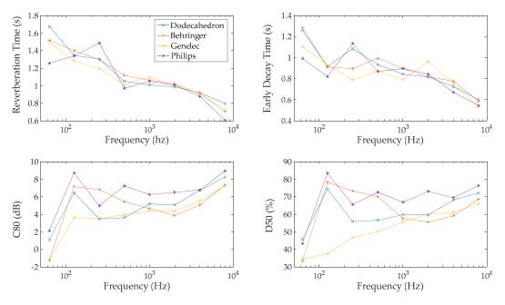
Figure 12. RT, EDT,  $C_{80}$  and  $D_{50}$  measured with different speakers.
