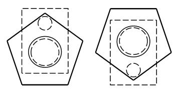
**Figure 3.** Placement of the face of the directional loudspeaker according to the placement of the face of the dodecahedron speaker (twelve positions measurements).
