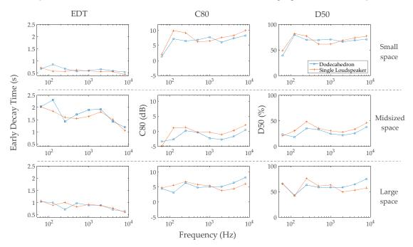
**Figure 7.** Early Decay Time (EDT), Clarity ( $C_{80}$ ) and Definition ( $D_{50}$ ) for the small, midsized and large space.
