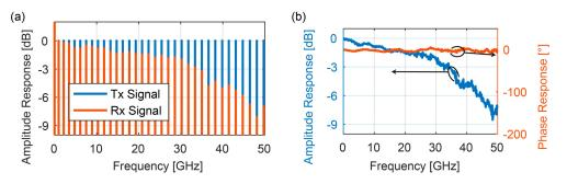
**Figure 3.** Characterization of frequency and phase response. (**a**) Amplitude spectrum of transmitted and received coarse non-integer spaced comb with a reduced set of 34 spectral lines. (**b**) Frequency and phase response measured with a comb of 331 spectral lines.
