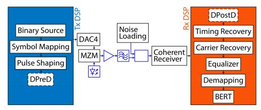
**Figure 5.** Overview of digital signal processing (DSP) and experimental set-up. The optical path is indicated by the blue color. Tx: transmitter; MZM: Mach–Zehnder modulator; Rx: receiver; BERT: bit error ratio testing.
