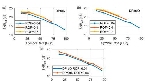
**Figure 7.** SNR improvement due to DPostD. Dependence of effective SNR on the symbol rate and ROF with DPreD (**a**) and with DPostD (**b**). (**c**) Comparison of effective SNR with an ROF of 0.04 with DPreD in blue and DPostD in red. The measured symbol rates are 14, 28, 56, 71, 80, and 96 GBd; QPSK was used as the modulation format.
