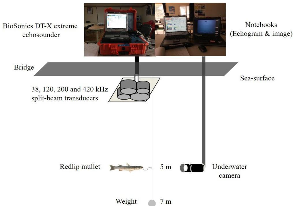
**Figure 2.** Experimental setup for the target strength (*TS*) measurements of Redlip mullet (*Chelon haematocheilus*) using a scientific echo-sounder (38, 120, 200, and 420 kHz).
