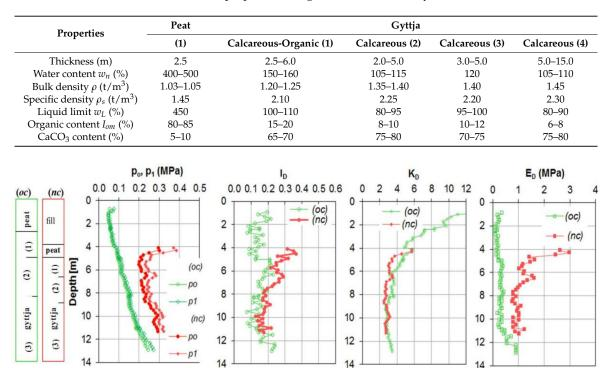
**Figure 2.** Profiles of the corrected readings  $p_o$  and  $p_1$  and index parameters  $I_D$ ,  $K_D$ , and  $E_D$  from dilatometer tests obtained for organic subsoil at the Koszyce site; (*oc*): overconsolidated subsoil, (*nc*): normally consolidated subsoil.
