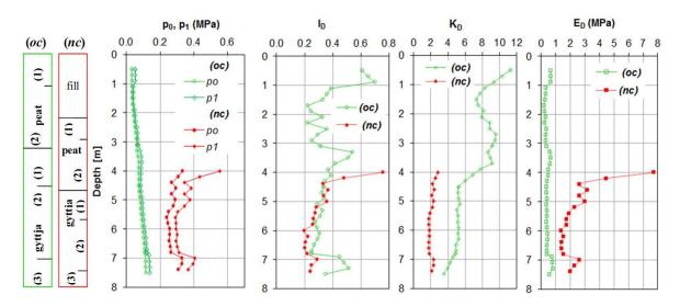
**Figure 1.** Profiles of the corrected readings  $p_o$  and  $p_1$  and index parameters  $I_D$ ,  $K_D$ , and  $E_D$  from dilatometer tests obtained for organic subsoil at the Antoniny site; (*oc*): overconsolidated subsoil, (*nc*): normally consolidated subsoil.
