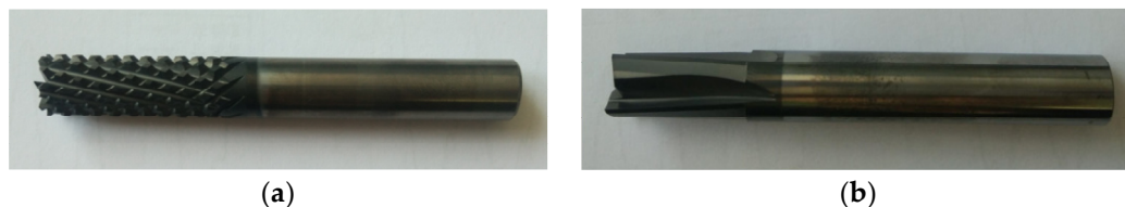
Figure 2. Two styles of milling cutter, (a) the rhombic milling cutter and (b) the staggered helical milling cutter.
