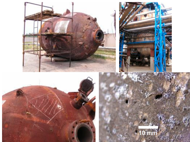
Figure 4. Breach of the cladding layer.
