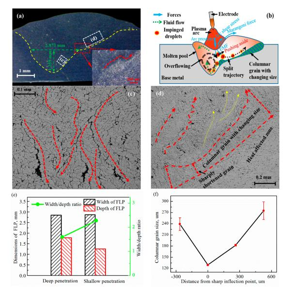
**Figure 4.** Welding torch inclined from the center line in the transverse section. (**a**) Molten pool profile; (**b**) schematic diagram of the molten pool behavior; (**c**) signs of downward flow; (**d**) signs of upward flow; (**e**) width, depth and width/depth ratio of the FLP; (**f**) columnar grain size along the upward wall.
