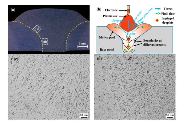
**Figure 2.** Welding torch perpendicular to the surface of the base metal in the transverse section. (a) Molten pool profile; (b) schematic diagram of the molten pool behavior; (c) columnar grain at the shallow level; (d) refined grain at the finger-like penetration (FLP) level.
