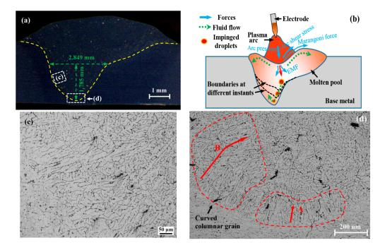
**Figure 3.** Welding torch inclined from the center line in the transverse section. (**a**) Molten pool profile with the sharp inflection point (SIP) not present on the non-impact action side (NIAS); (**b**) schematic diagram of the molten pool behavior; (**c**) columnar grain on the NIAS in the FLP level; (**d**) shortened columnar grain on the impact action side (IAS) at the shallow level.
