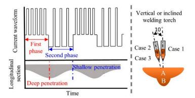
**Figure 1.** Schematic diagram of the current waveform and longitudinal sections of the double pulsed-gas metal arc welding (DP-GMAW) weld pool and the inclination of the welding torch.
