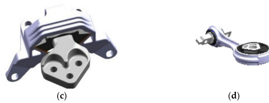
Figure 5. (a) Powertrain with highlight of support positions: (b) engine bracket; (c) gearbox bracket; (d) differential bracket.
