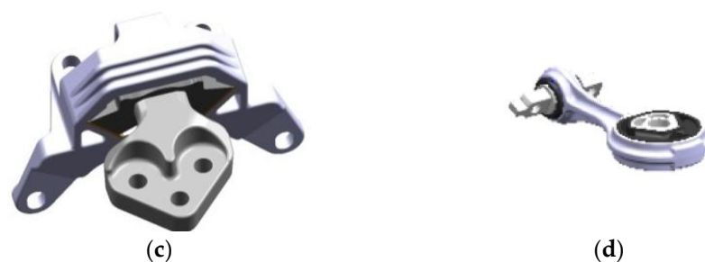
Figure 5. (a) Powertrain with highlight of support positions; (b) engine bracket; (c) gearbox bracket; (d) differential bracket.
