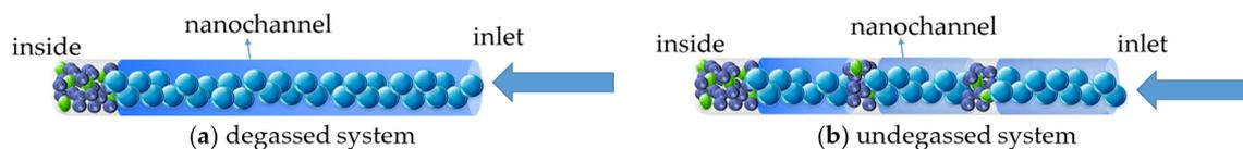
**Figure 7.** Cartoon of status of gas liquid in a nanochannel of degassed and undegassed systems. (
