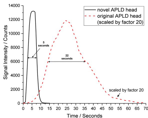
**Figure 2.** Compared smoothed desorption from spots with about 1.5  $\mu\text{g}$  Tetryl. Measured at negative CI mode and fragment  $m/z$  241. Novel system with short transferline and heated APLD head (solid line). Original measurement system with long transferline (dashed line). Compared is the full width at half maximum.
