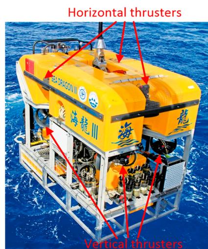
**Figure 1.** The Sea Dragon remotely operated vehicle (ROV) at sea.
