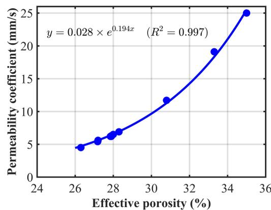
Figure 7. Effective porosity vs. permeability.
