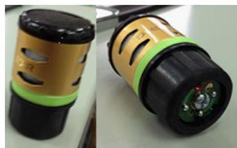
**Figure 9.** TS-5 type moving-coil microphone.
