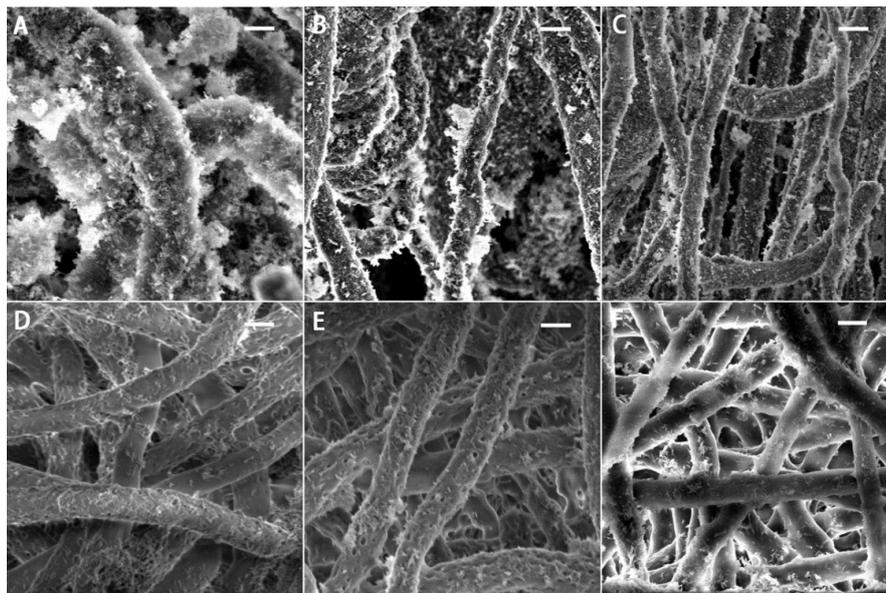
**Figure 6.** SEM of PDLLA/nHA composite fibrous membranes with different nHA content. Scale bars represent 1  $\mu\text{m}$ .
