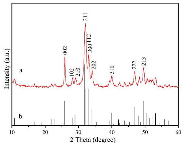
**Figure 3.** XRD of nHA particles, (a) self-made sample; (b) standard card.
