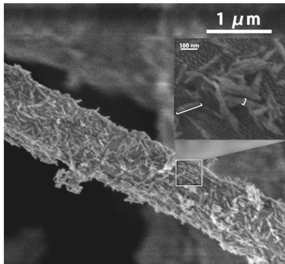
**Figure 4.** SEM of PDLLA/nHA composite fibers and partially enlarged detail.
