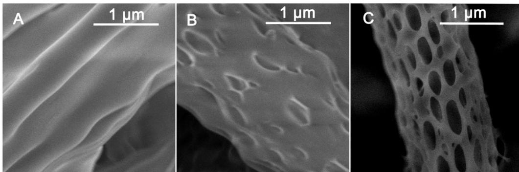
**Figure 2.** SEM of PDLLA fibers electrospun with different temperature under 80% humidity, (A) 15 °C; (B) 20 °C; (C) 25 °C.
