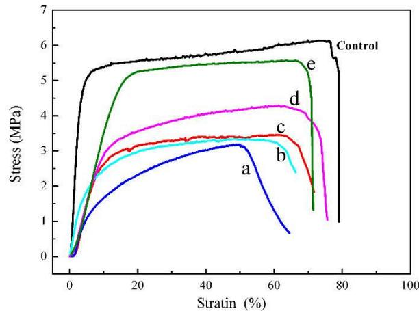
**Figure 8.** Tensile test of PDLLA/nHA composite fibrous membranes.
