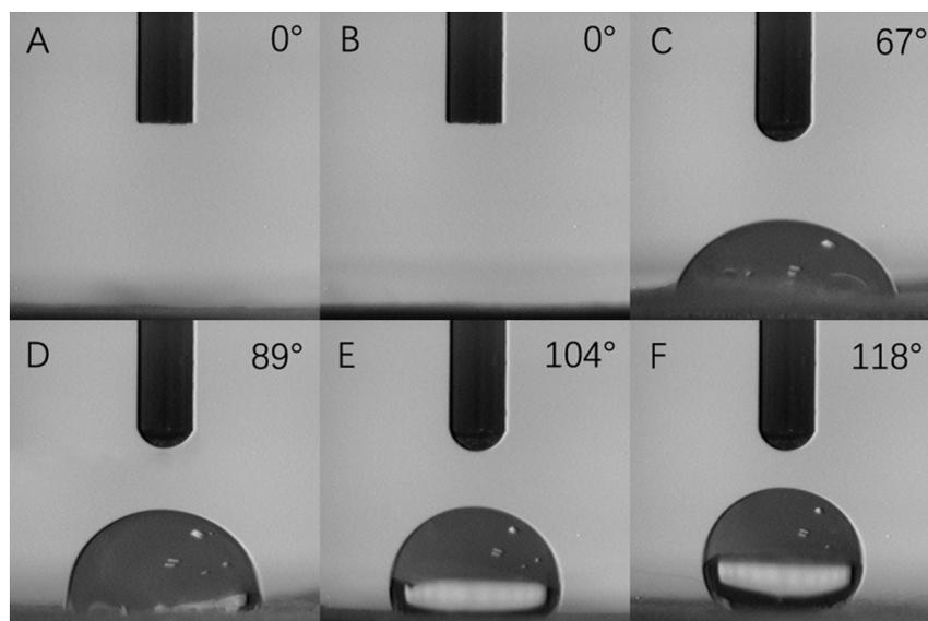
**Figure 7.** WCA of PDLLA/nHA membranes with different content of nHA, (A) 11.2%; (B) 10.6%; (C) 8.8%; (D) 5.5%; (E) 4.1% and (F) Control group.
