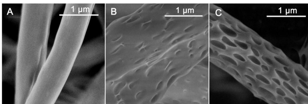
**Figure 1.** SEM of PDLLA fibers electrospun with different humidity at 25 °C. (A) 50%; (B) 65%; (C) 80%.
