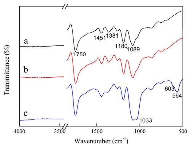
**Figure 5.** FTIR of (a) porous PDLLA membrane; (b) porous PDLLA membrane shrank in absolute ethyl alcohol; (c) PDLLA/nHA composite fibrous membrane.
