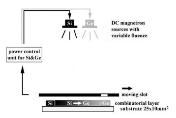
**Figure 1.** Set-up used for the combinatorial deposition of the a-Si<sub>1-x</sub>Ge<sub>x</sub> layer.
