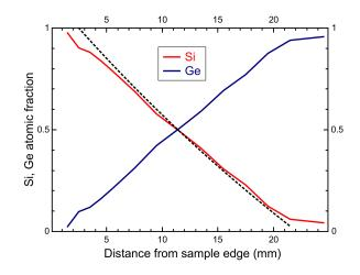
**Figure 2.** Atomic fraction as a function of position along the center line of the combinatorial sample measured by Rutherford backscattering spectrometry. The black dotted line shows the distribution of the atomic fraction based on the calibration using energy dispersive spectrometry (EDS) in a scanning electron microscope.
