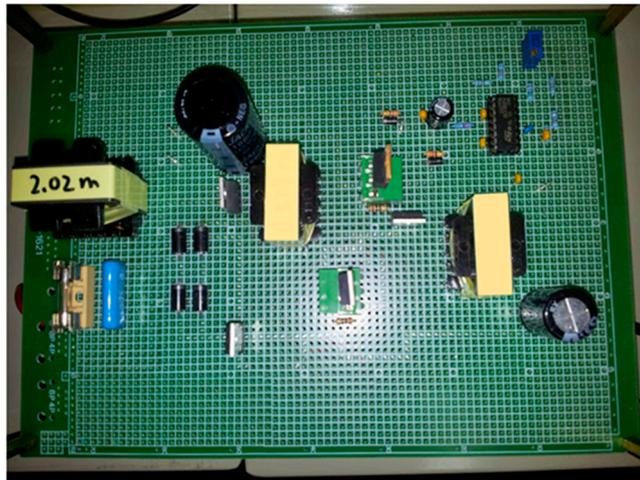
Figure 9. The prototype LED driver.
