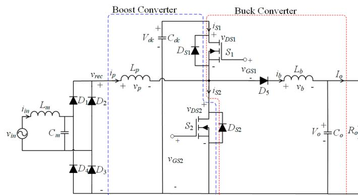
Figure 1. An integrated circuit with a boost converter and buck converter [12].
