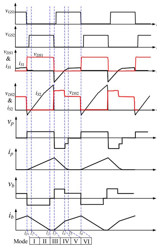
Figure 4. Theoretical waveforms.
