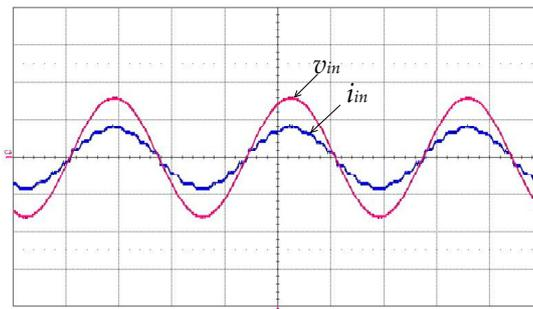
Figure 5. Waveforms of the input voltage and current. ( $v_{in}$ : 100 V/div,  $i_{in}$ : 1 A/div, time: 5 ms/div).
