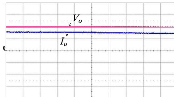
Figure 7. Waveforms of  $V_o$  and  $I_o$ . ( $V_o$ : 100 V/div,  $I_o$ : 0.2 A/div, time: 5 ms/div).
