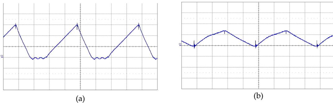
Figure 6. Waveforms of inductor currents (a) Buck-boost inductor current  $i_p$  ( $i_p$ : 1 A/div, time: 5  $\mu$ s/div) and (b) Buck inductor current  $i_b$  ( $i_b$ : 0.5 A/div, time: 5  $\mu$ s/div).
