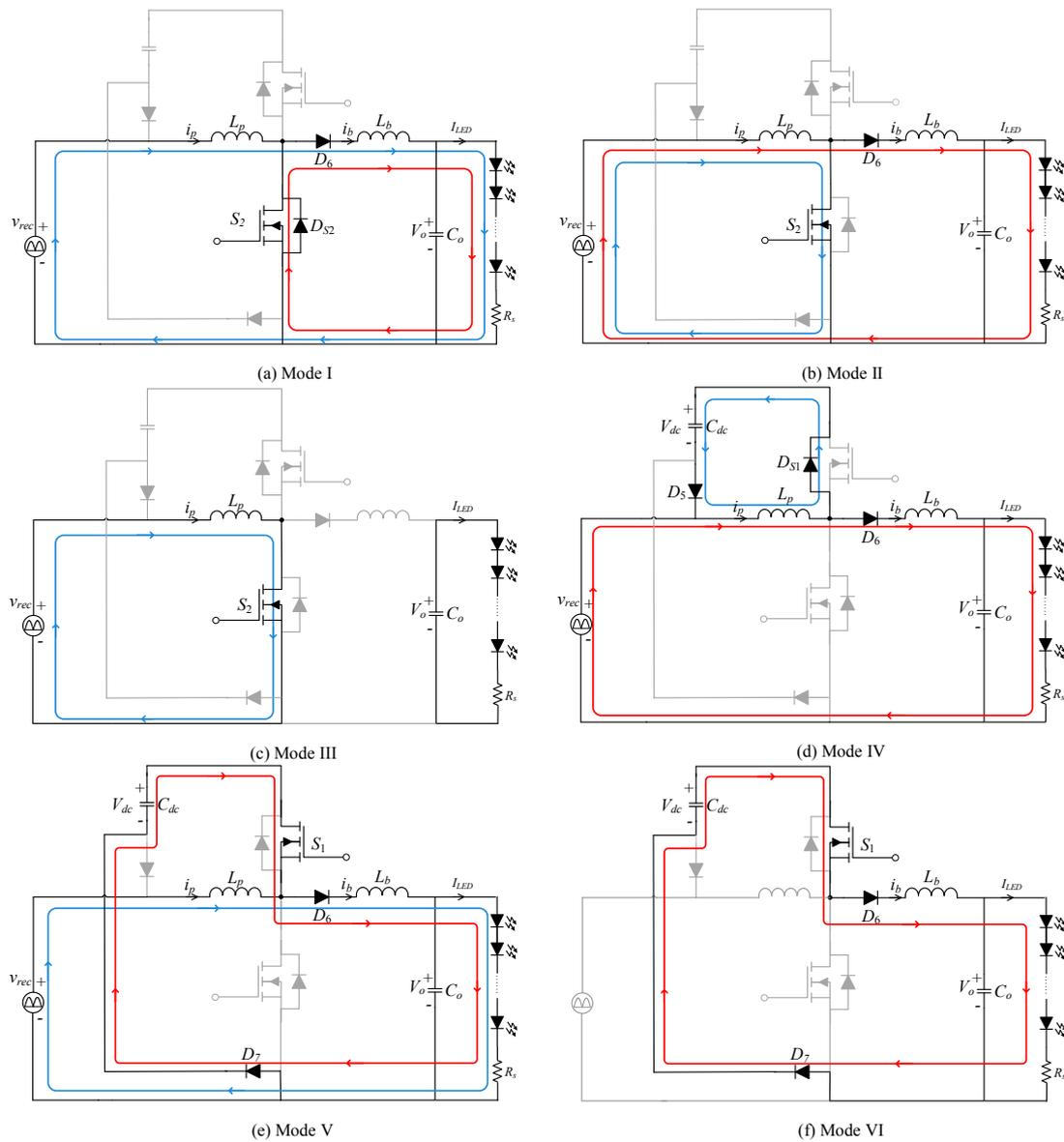
Figure 3. Equivalent circuit of operation modes: (a) Modes I–(f) Modes VI.
