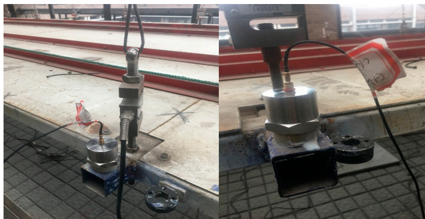
(b) Accelerometer attached close to cable.
