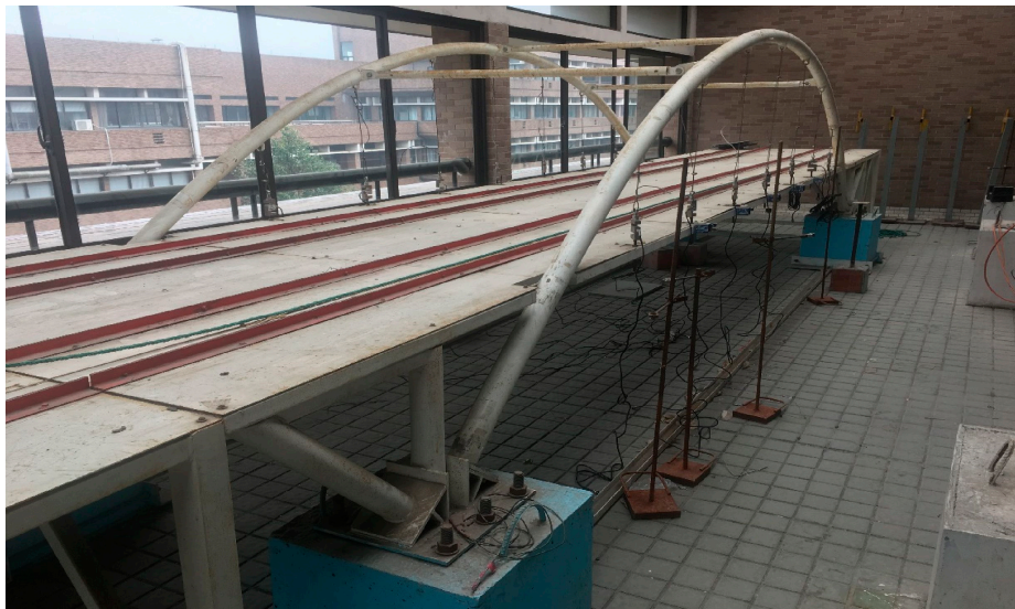
Figure 7. The arch cable bridge lab model built at Zhejiang University Laboratory.
