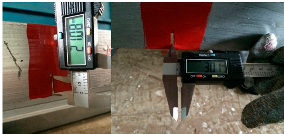
Figure 6. A general view of the crack. The right photo shows the width of the crack (around 0.003 m), and the left photo shows the height of the crack for \delta = 30\% ( 0.072 \times 0.3 = 0.0216 \text{ m} \approx 0.021 ).
