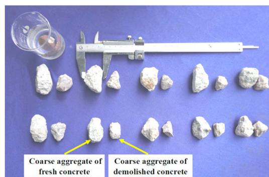
**Figure 2.** Maximum aggregate sizes for fresh concrete and demolished concrete.
