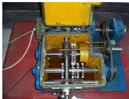
Figure 22. Fault simulation device for rolling bearing and gear. 1—motor, 2—coupler, 3—replaceable rolling bearing with 6207, 4—belt pulley, 5—device box, 6—transmission shaft, 7—gear.
