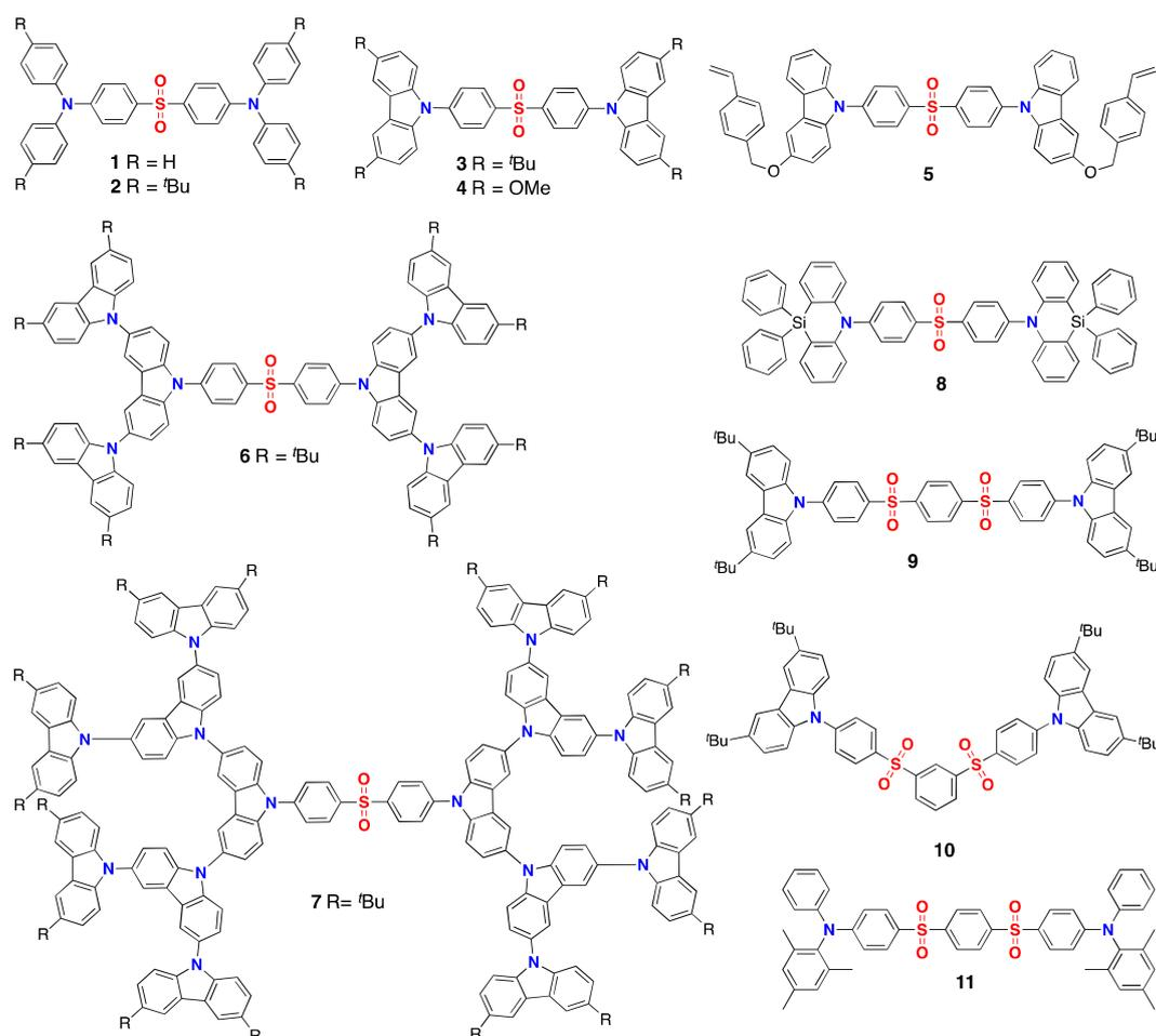
**Figure 2.** Diphenylsulfone-based (1–8) and bis(phenylsulfonyl)benzene-based (9–11) emitters.
