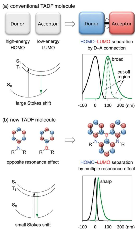
**Figure 7.** Comparative representation of energy diagram for a traditional TADF emitter (a) and the design developed to generate a multiple resonance effect (b). The curve corresponding to the emission spectrum of a benchmark blue OLED is provided as the green dotted line. Figure reproduced with permission from Hatakeyama et al. [95] (reproduced with permission from [95] Copyright Wiley-VCH, 2016).
