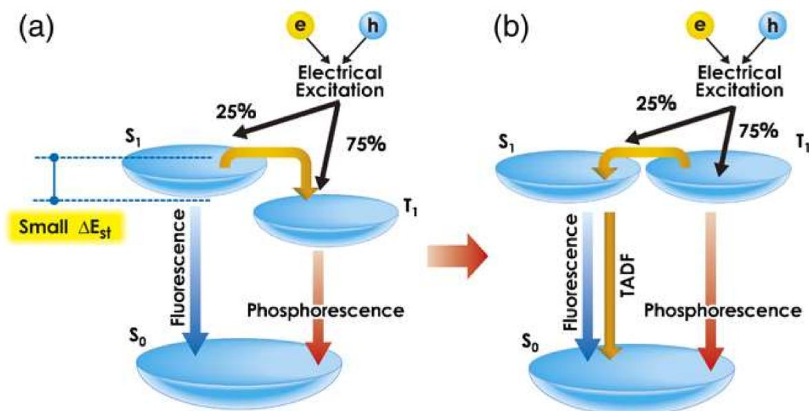
**Figure 1.** Light generation processes in (a) fluorescence and phosphorescence-based organic light-emitting diodes (OLEDs) and (b) thermally activated delayed fluorescence (TADF)-based OLEDs. Figure reproduced with permission from Adachi et al. [54] (reproduced with permission from [54]. Copyright The Japan Society of Applied Physics, 2014).
