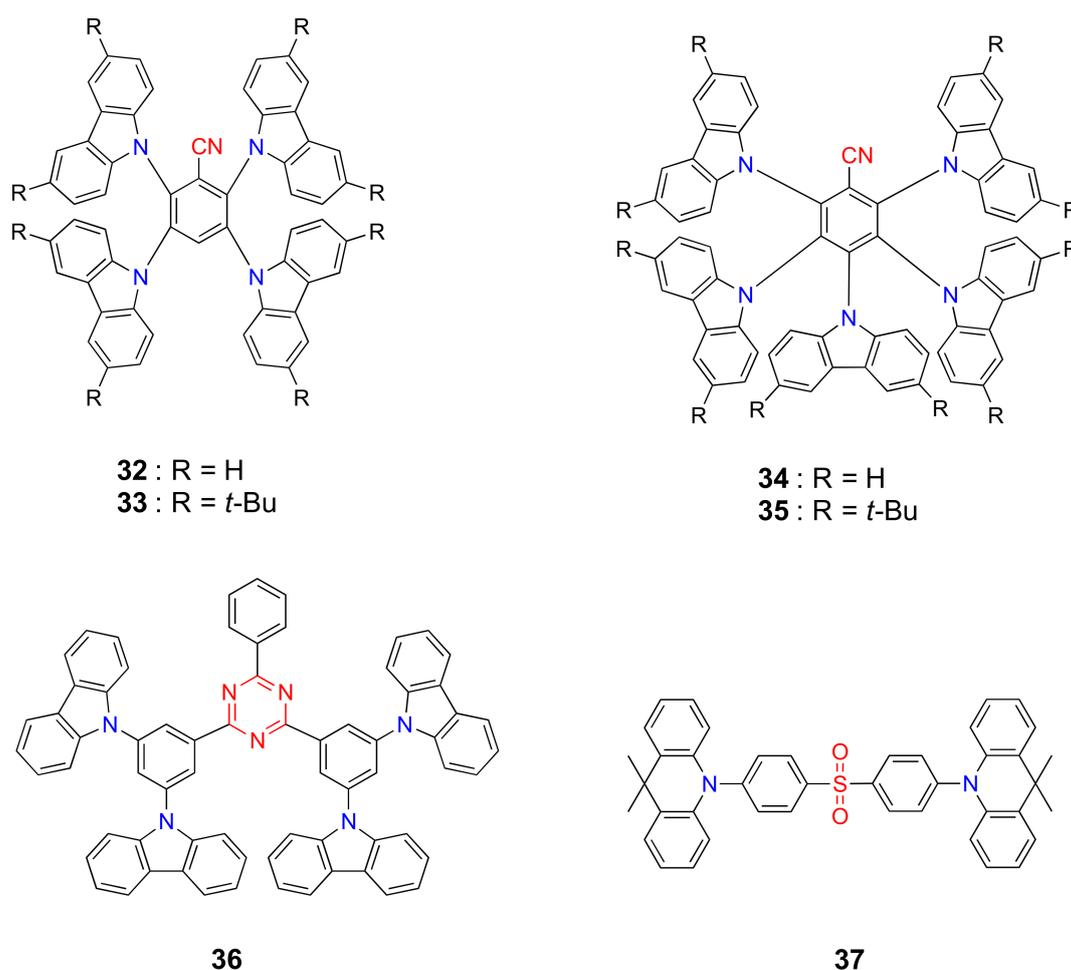
**Figure 10.** TADF emitters examined for the device lifetime.
