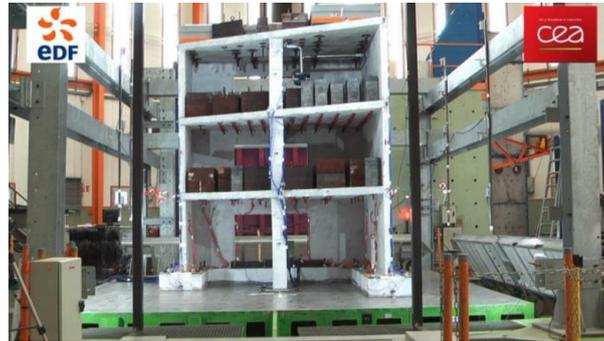
**Figure 1.** The asymmetric three-storey reinforced concrete building used for the SMART (Seismic design and best-estimate Methods Assessment for Reinforced concrete buildings subjected to Torsion and nonlinear effects) 2013 international benchmark campaign.
