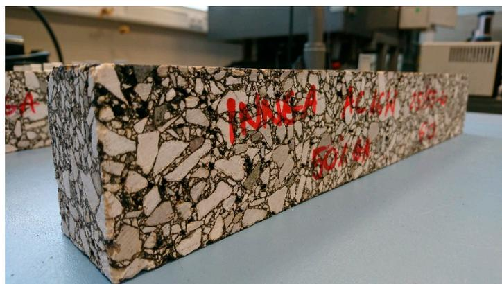
**Figure 2.** Beam for four-point bending beam test (4PB) fatigue and stiffness test.
