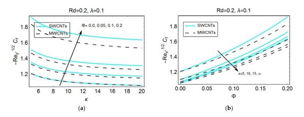
**Figure 6.** Skin friction coefficient for some values of: (a)  $\Phi$ ; and (b)  $\kappa$ .
