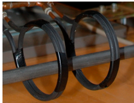
Figure 7. Helmholtz coil with a wire, for which the results are shown in Figure 8.
